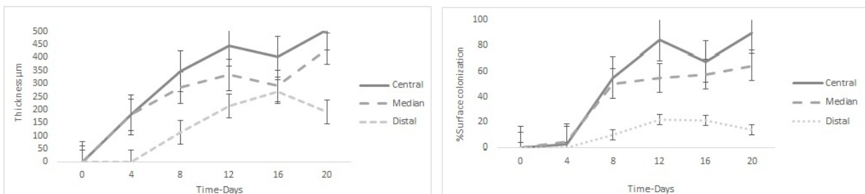
Figure 1. Percentage of thickness of Alternaria alternata biofilm growth on tuffa tiles (left), surface colonization on tuffa tiles (right); points: central (—), median (- - -), distal (· · ·).
